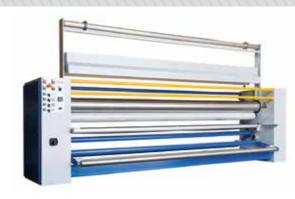
The beltless calender type GFC is designed for the fixation of dispersed dyes and pigments printed directly on the material. Flags, banners and backlit material are ideal to be processed on this type of calender. The stable temperature thanks to the thermal oil and electrically heated drum will give you consistent brilliant colours. Tension of the substrate at the infeed and outfeed is very well controlled by means of special weights that keep the substrate from moving.
